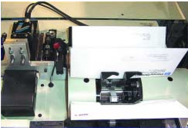
An IntegraVision MaxRead 3 mounted on the output of an inserter for inline mail sorting.
