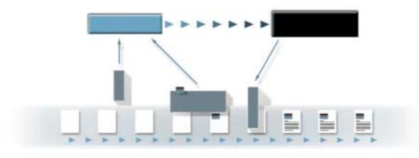
By reading a unique identifier on a personalised mail piece or secure document, the relevant address or other variable data can be located within a database and printed on the correct piece at the appropriate time.
