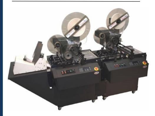
The Ameritek Tabber can also be configured as a Dual Headed Tabber. This system can tab on the leading (toe) and trailing (heel) edges of a booklet in a single pass. The Dual Headed Tabber can run in-line or off-line as a system, or the Tabbers can be unlocked and used as stand-alone units.
