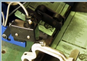
Feeder timing controlled by holding down ski arm triggering micro-switch.
